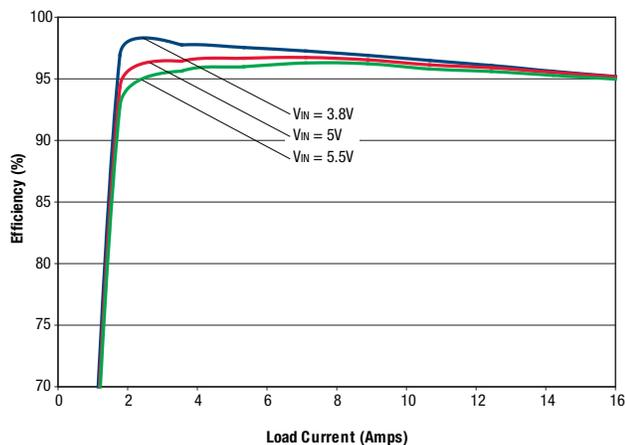
OKX-T/16-W5 Efficiency vs. Line Voltage and Load Current @ +25°C
