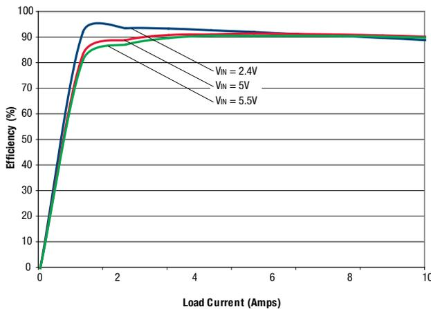
OKX-T/10-W5 Efficiency vs. Line Voltage and Load Current @ +25°C
