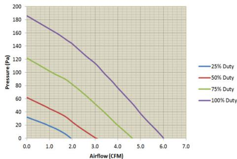
D1U54T-W-800-12-HB4C P-Q Airflow (back to front air direction)
