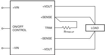
Figure 7. Trim Connections To Increase Output Voltages Connect sense to its respective Vour pin if sense is not used with a remote load.
