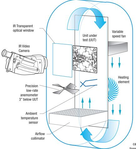
Figure 10. Vertical Wind Tunnel
