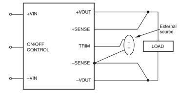
Figure 9. Trimming with an External Source
