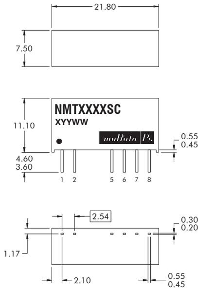
All dimensions in mm  $\pm 0.25$ mm. All pins on a 2.54 pitch and within  $\pm 0.25$  of true position. Weight: 3.85g
